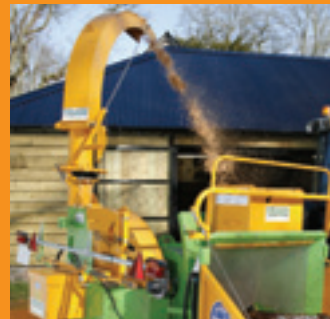
The Heizohack drum chipper producing a consistent biomass quality chip.
